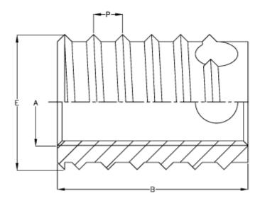
Female thread A = M16 Length B = 14 Male thread E = 20.0 Min hole depth blind hole = 17
